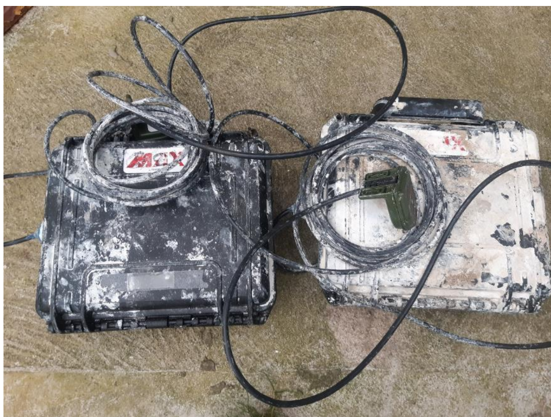
Figure 3.1 Equipment in returned state. The weatherproof cases were heavily fouled by bird guano.
